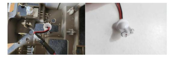
5. Once tested, Mount the new led panel over the mounting points and use the glue supplied to glue the 3 mounting points down. Repeat this on the other led panel.
