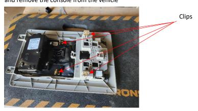
2. Once the panel is removed, Split the black section from the cream section. There are 2 tabs at the front of the panel (front windscreen side) once pushed in the black panel will drop down at the front and unhook at the back
